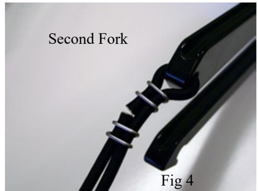
**Step 5: Crimp hog ring on first fork.** Before crimping the hog ring, make sure the cord is evenly distanced between the forks. This is done by pulling the cord in the middle until even loops are achieved between both forks. See **Fig-5**.
