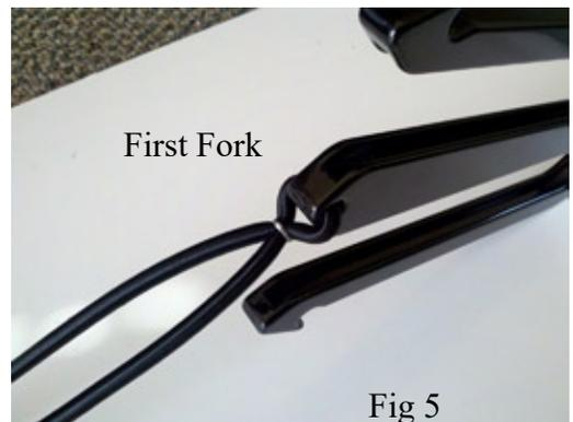
**Step 4: Heat Shrink tube.** Slide one heat shrink tubing over the crimped area (near the tip of the fork) and apply even heat to shrink the tubing. **BE CAREFUL not to burn the shock cord as it will melt.** Slide the second tubing over the first and shrink again. Repeat for other side. See **Fig-6**.
